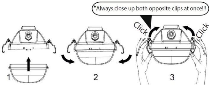
close clips symmetrically from the middle to the side of the luminaire
